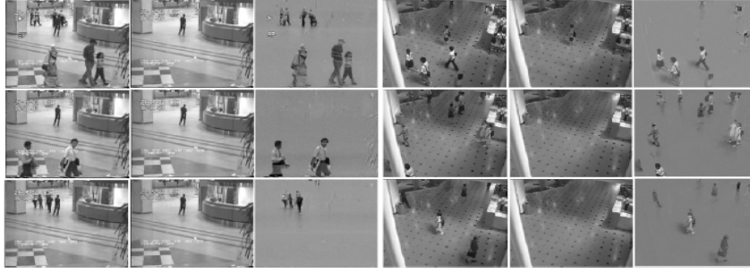
Figure 4.7: Background subtraction in surveillance video. Images in columns 1 and 4 are frames of the video sequence of an airport and a shopping mall, respectively. Images in columns 2 and 5 are recovered backgrounds \hat{\mathbf{L}} , and columns 3 and 6 correspond to foregrounds \hat{\mathbf{S}} by the ALM-SOR-SVD method.
