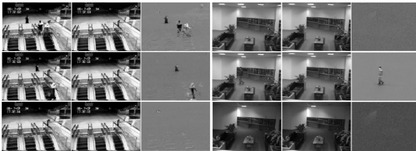
Figure 4.8: Background subtraction in surveillance video. Images in columns 1 and 4 are frames of the video sequence of an escalator and an office, respectively. Images in columns 2 and 5 are recovered backgrounds \hat{\mathbf{L}} , and columns 3 and 6 correspond to foregrounds \hat{\mathbf{S}} by the ALM-SOR-SVD method.
