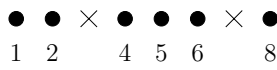
Figure 2.3: Generic NLA with N = 6 sensors (filled black circles) and 2 empty locations (crosses)
